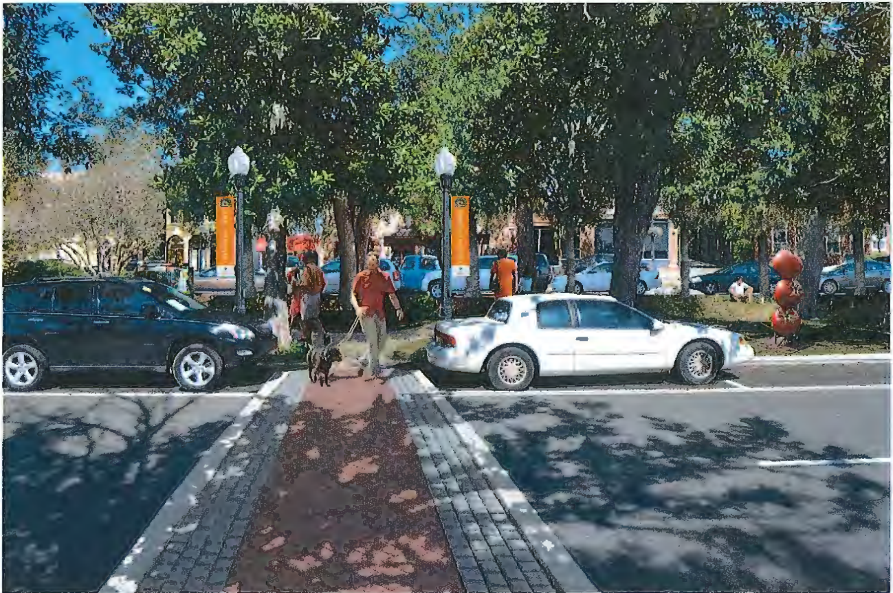
Proposed Conditions: Clearly delineated crosswalks should be installed at regular intervals along the parkways for pedestrian safety. All pedestrian access points into the parkways should be framed by dual light poles that illuminate the entry and feature parkway banners. The under canopies of the trees should be limbed up to approximately 12' and low shrubs should be kept below 3'. It is recommended that simple, meandering pathways be installed within the parkways to promote walking in a park-like setting. Populate each parkway as desired with animation treatments such as benches, swings, sculpture, interactive art, water features, games, etc.
